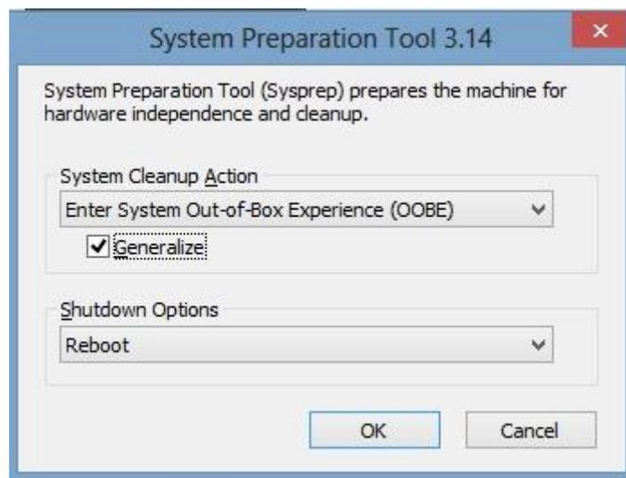
**Figure 23: System Preparation tool**
